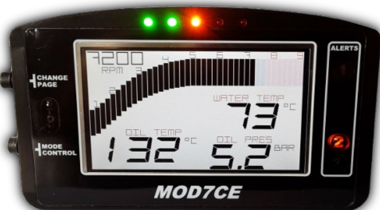
Example of the display in day mode (white background) in 3 functions mode (without gear box indicator)
