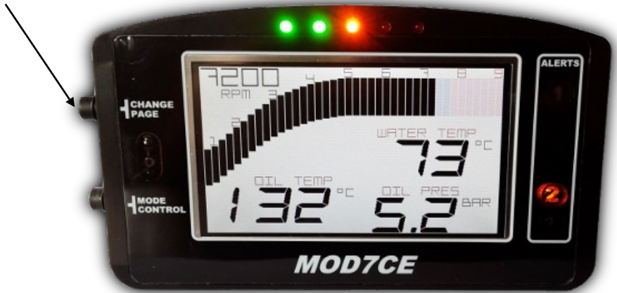
Example of the display in day mode (white background) in 3 functions mode (without gear box indicator)
